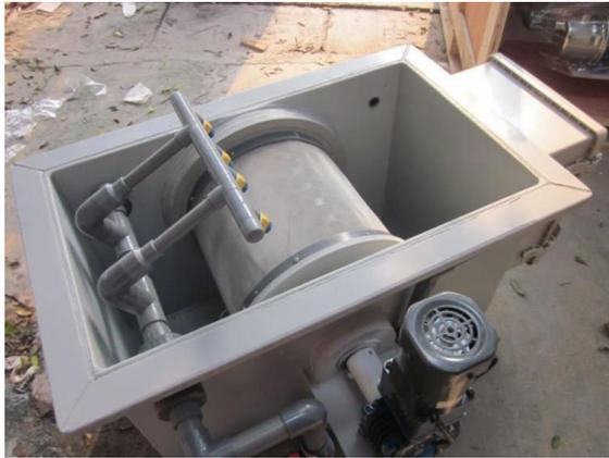
Gambar 1 Mesin rotary drum filter
