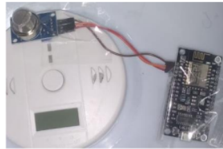
Figure 5. MQ135 AND NODEMCU SENSOR CONNECTION
