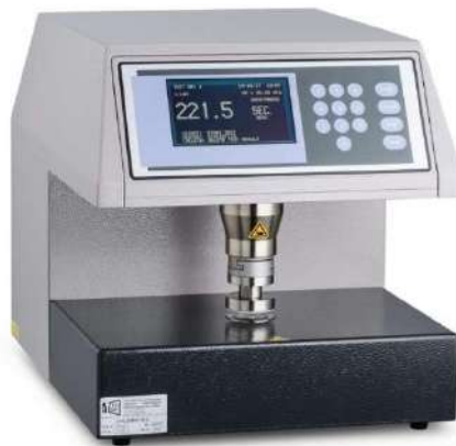
Gambar 3 Bekk Smoothness Tester
