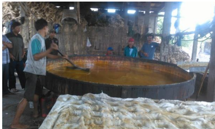
Fig. 5. Cooked sugarcane juice, stirred and ready for molding
