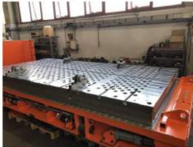
Gambar 2.4 Moving bolster Sumber: c.v.c, 2024
