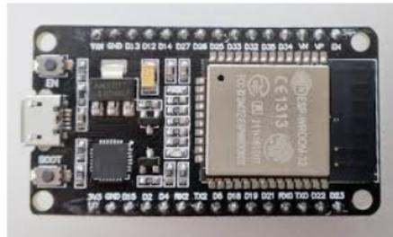
Gambar 2. 1 Modul Esp32
