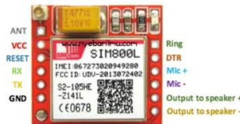
Gambar 2. 2 Gambar Modul GSM
