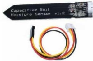
Gambar 2.1 Sensor Moisture Soil
