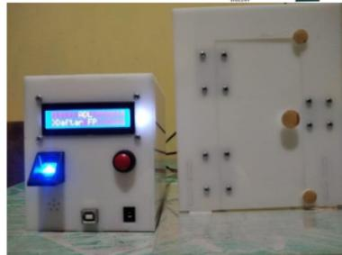
Gambar 4.2 Alat Smart Lockdoor berbasis Arduino Mega
