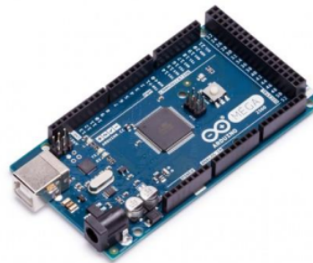
Gambar 2.1 Board Aduino Mega
