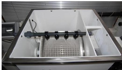
Gambar 2. 1 Mesin *Rotary Drum Filter*
