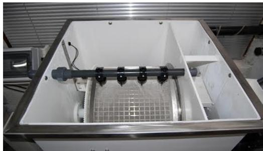
Gambar 2. 1 Mesin *Rotary Drum Filter*
