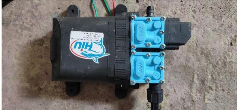
Gambar 4.2 Motor *Sprayer*
