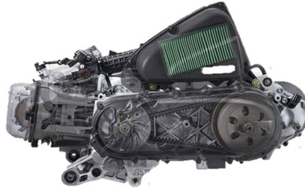
Gambar 2. 1 Mesin Motor Matic 110CC
