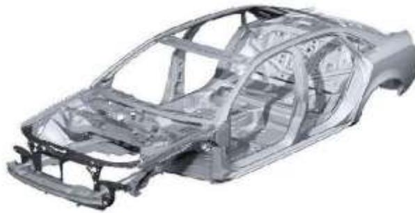
Gambar 2.4 *Chassis Monocoque Frame*
