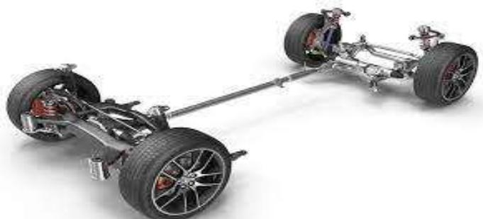
Gambar 2.5 *Chasis Backbone Frame*
