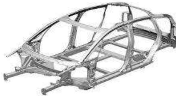
Gambar 2.6 Chasis Aluminium Space Squere
